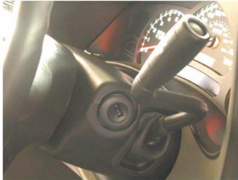
Stabilize the scene by addressing the hazards. Secure the vehicle prior to vehicle entry. Ensure that: the transmission is in Park or Neutral, the parking brake is applied, the ignition is off, the key is removed, and the wheels are chocked (blocked) in some way so that there is no other means by which the vehicle can become mobile.
