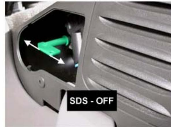
Disconnects 42 volt battery from vehicle electrical system:
