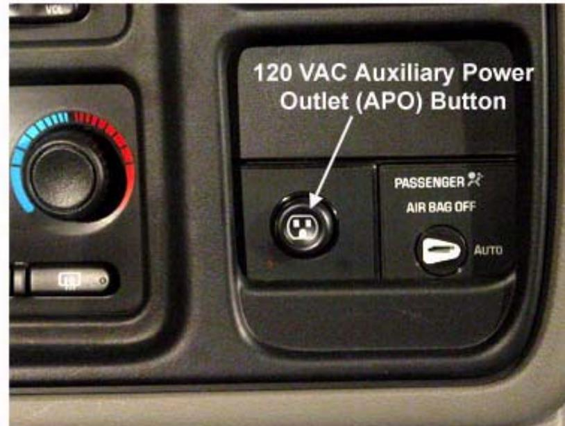
**120 VAC Auxiliary Power Outlet (APO) Button** – The main control of the 120 volt system is located to the right of the heating, vent and air conditioning controls in the center of the instrument panel.
