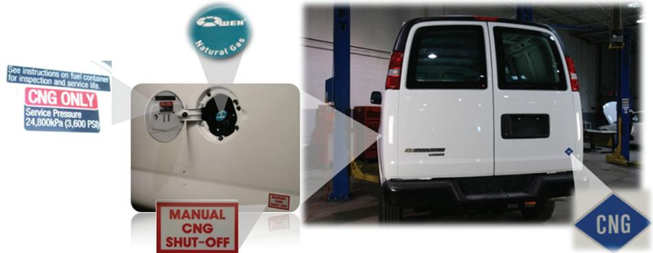
The CNG labels inside of the vehicle are located on:
