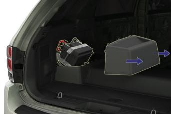
After disabling 12 volt power, WAIT a minimum of 10 seconds to allow any undeployed air bag reserve energy and high voltage energy to dissipate before cutting into the vehicle.
