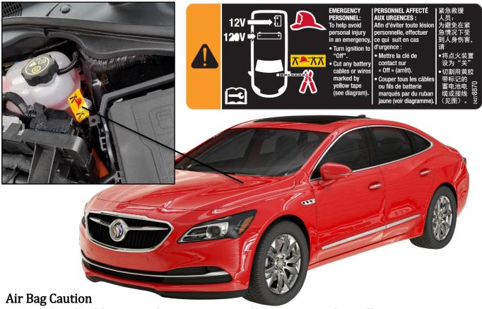
After disabling 12 volt power, wait at least 10 seconds to allow any un-deployed airbag reserve energy to dissipate.
