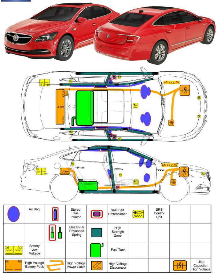
The Buick LaCrosse with eAssist technology incorporates a low voltage battery that must be disconnected prior to occupant extrication.
