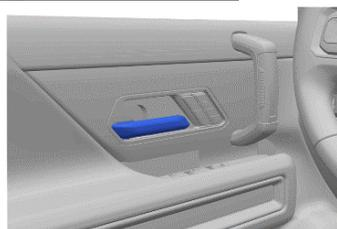
If the doors remain locked, pull **twice** on the inside door handle to gain access to the occupant.
