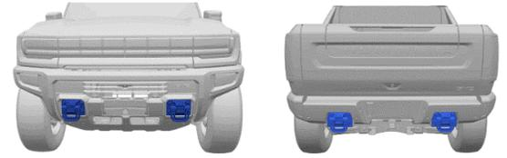
General Motors recommends a flatbed carrier to transport a disabled vehicle. A wheel lift truck along with properly rated tow dollies can be used if a flatbed carrier is not available.
