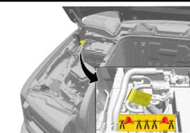
Airbags can be disabled by removing the 12v battery negative cable. This will disable the thermal runaway alert and mitigation.
