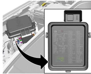
If the horn must be disabled prior to transport, locate and remove the horn fuse from the underhood electrical center.
