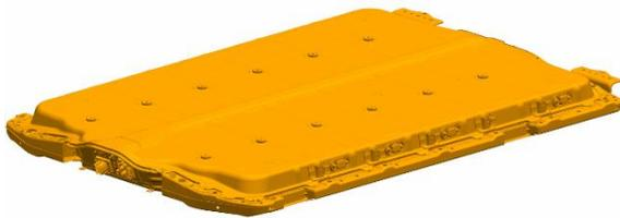
The battery is a High Voltage (Class B) Li-ion pack, that is a mounted under the vehicle and is a structural part of the floor pan.
