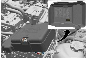
If the horn must be disabled prior to transport, locate and remove the horn fuse from the underhood electrical center.
