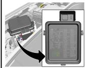
If the horn must be disabled prior to transport, locate and remove the horn fuse from the underhood electrical center
