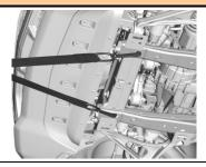
General Motors recommends a flatbed carrier to transport a disabled vehicle. A wheel lift truck along with properly rated tow dollies can be used if a flatbed carrier is not available.
