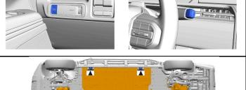
Do NOT lift the vehicle from any locations on the high voltage battery.
