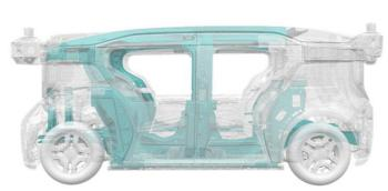
The passenger compartment is protected using high strength steel in the forward structure, roof headers, body pillars, rocker panels, door reinforcement beams, and floor structure.
