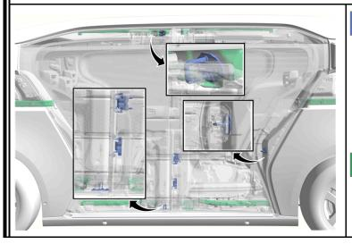
The sliding door latching system has three striker points;
