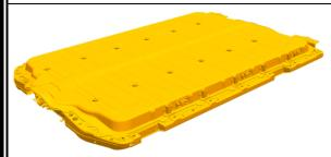
The battery is a High Voltage (Class B) Li-ion pack, that is a mounted under the vehicle and is a structural part of the floor pan.
