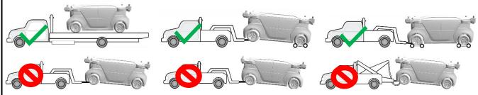
Moving the vehicle with the drive wheels on the ground will generate unwanted energy. Limit the movement of the vehicle to the distance required to prepare the vehicle for towing.
