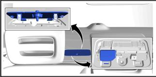
If the front compartment panel electric release is not available, a manual release lever is located in the front package shelf area of the vehicle.
