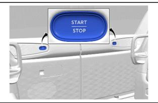
Press one of the Start/Stop buttons, located on any of the left or right-side doors to disable vehicle propulsion.
