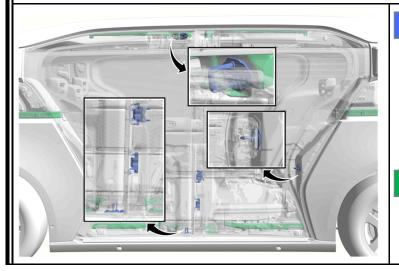
The sliding door latching system has three striker points;
