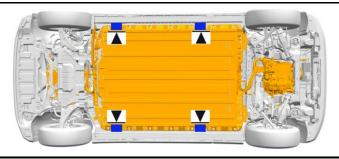
There are features on the body of the vehicle, for use as primary lifting points.
