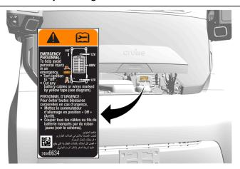
The battery warning label is located on the left side of the front compartment.
