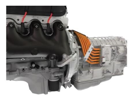
**Conventional Engine with an Electronically Variable Transmission (EVT)**
