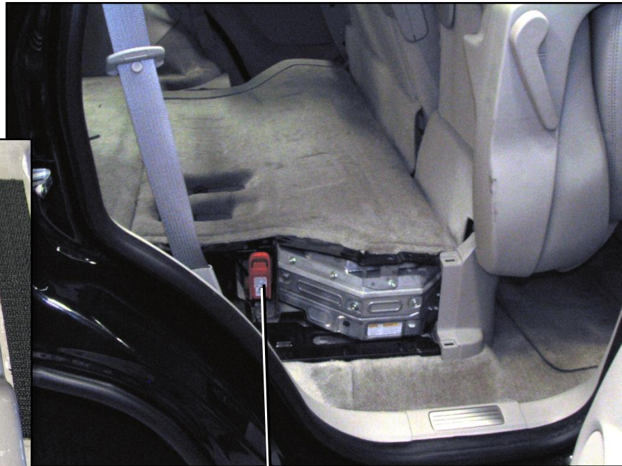
300V Hybrid Battery Manual Disconnect
